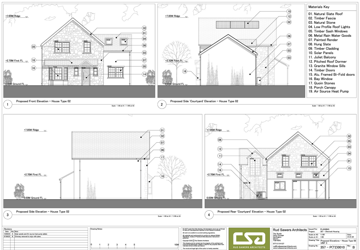
Proposed elevations - house type 2
