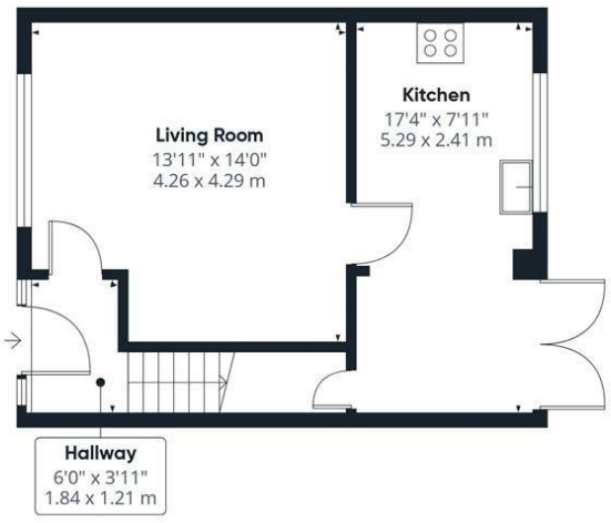
Ground floor Building 1
