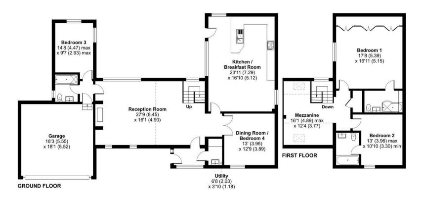
Floor plan produced in accordance with RICS Property Measurement 2nd Edition, Incorporating International Property Measurement Standards (IPMS2 Residential). © ntchecom 2025. Produced for Strakers. REF: 1228630
