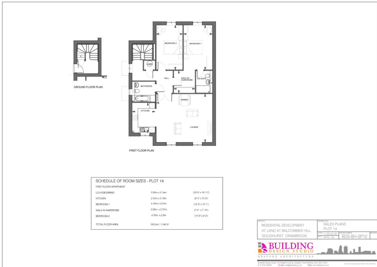
Architectural floor plan and room schedule - Plot 14 - Not to scale
