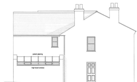
PROPOSED WEST ELEVATION 1:50 @ A2
