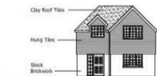
Proposed North-West (Front) Elevation Scale 1:200
