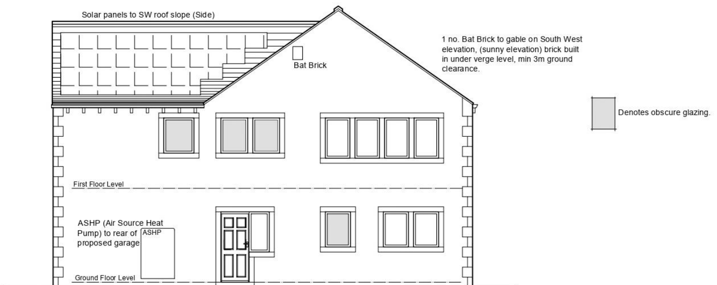
South West Elevation (side)
