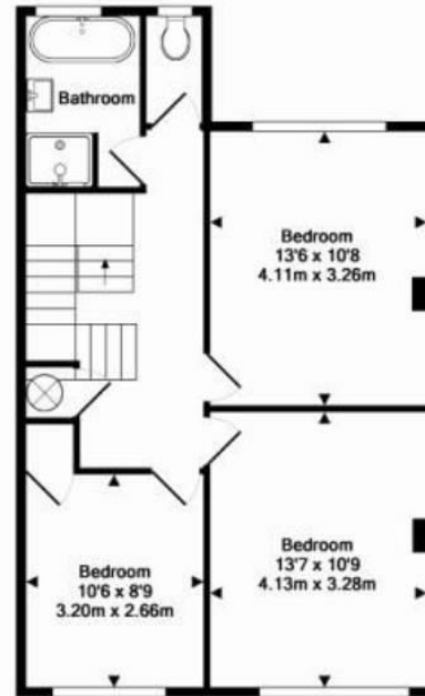
1ST FLOOR APPROX. FLOOR AREA 595 SQ.FT. (55.3 SQ.M.)
