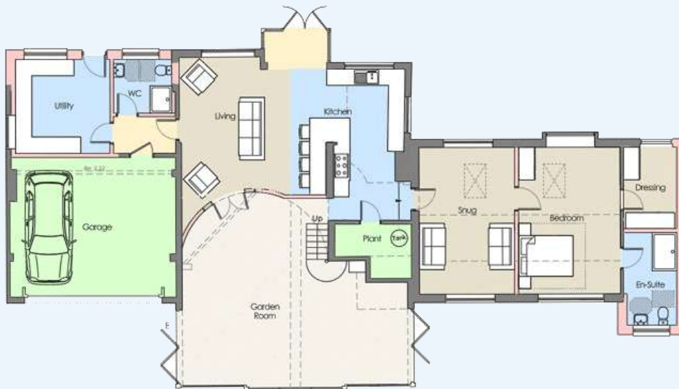
Proposed new ground floor plan
