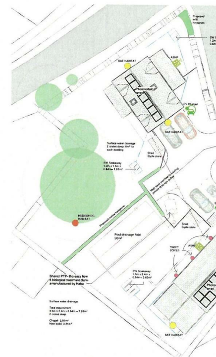
Site plan- Drainage, ecology and lands 1 : 200
