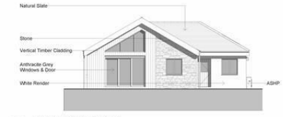
2 Elevation 2 - North Elevation 1:100
