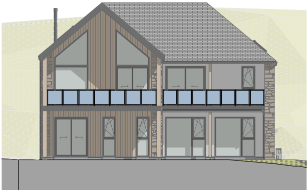
E-02 South Elevation 1:100
