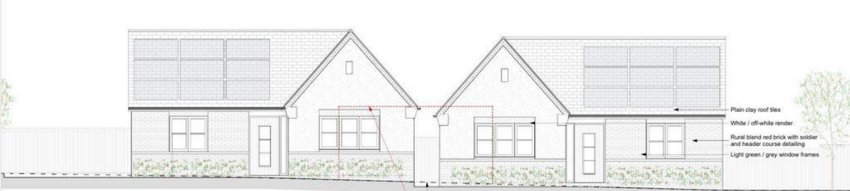
Rear Elevation - North Facing SCALE: 1:50
