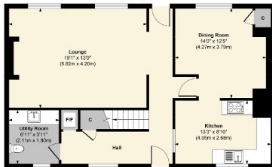
Ground Floor Approximate Floor Area
