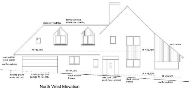
North West Elevation
