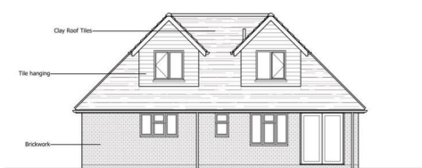
Proposed Side Elevation Scale 1:100
