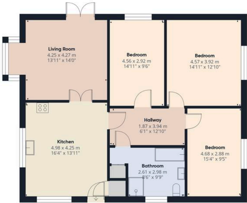
Ground Floor Building 1
