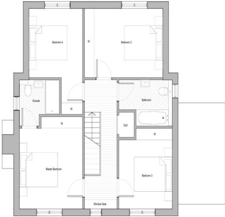
Proposed First Floor Plan Scale 1:50
