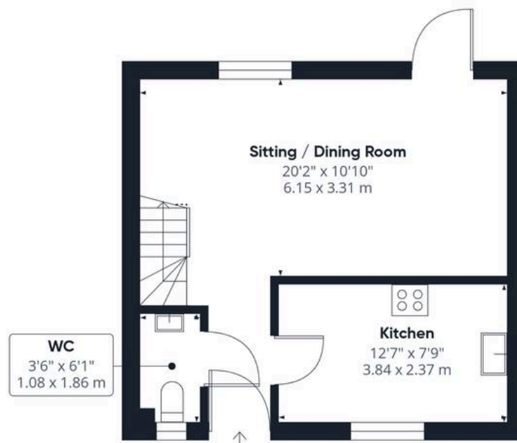
Ground Floor Building 1
