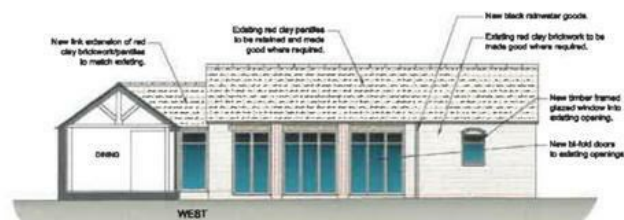
Proposed Elevations - Farmhouse & Barn 1 scale 1:100 @ A1
