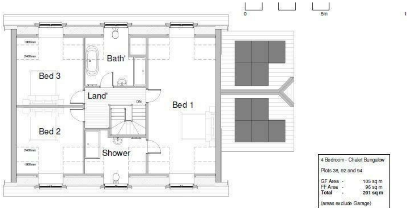
2 First Floor Plan 1 : 100
