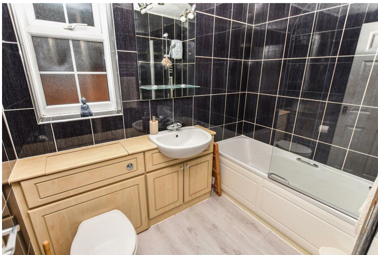
Window to flank, fully tiled walls, chrome towel radiator, panelled bath with hand grips and electric shower over, shower screen, vanity wash hand basin with mixer tap and cupboards under, close coupled wc with concealed cistern and push button control.
