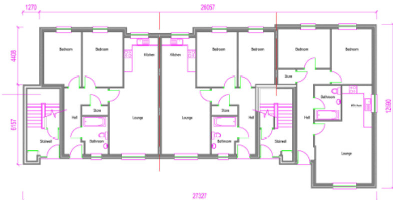
Ground floor Plan 1:100
