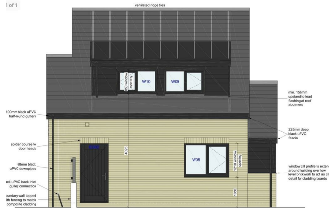
South-West Elevation (Side)
