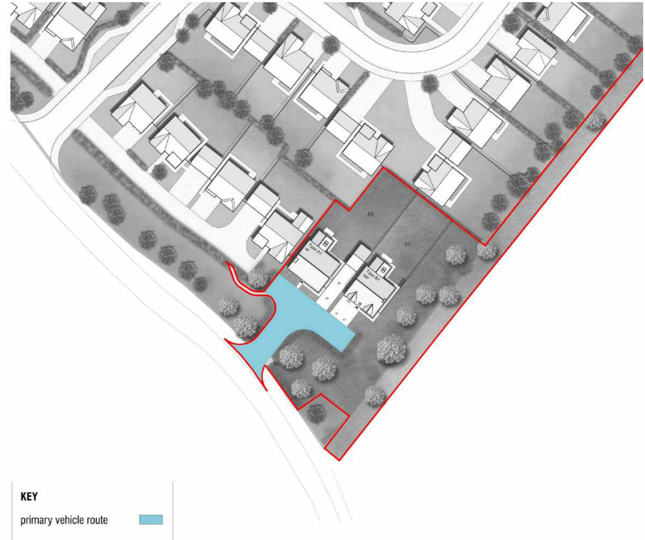
Movement Diagram showing street types, points of access and connections throughout the site and into the wider locality
