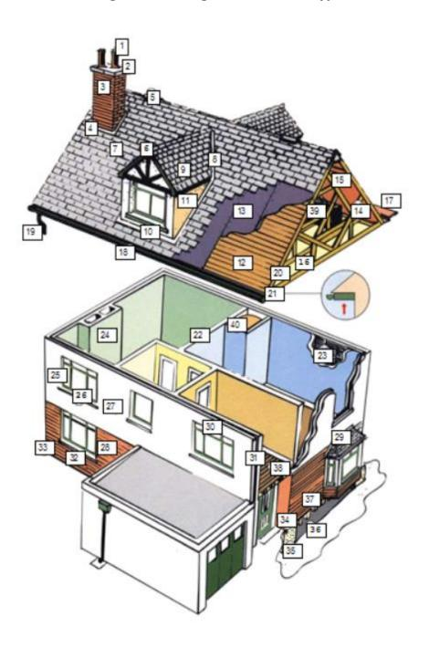
Chimney pots Coping stone 3 Chimney head 4 Flashing Ridge ventilation 5 Ridge board Slates/tiles 8 Valley guttering 9 Dormer projection 10 Dormer flashing 11 Dormer cheeks 12 Sarking 13 Roof felt 14 Trusses 15 Collar 16 Insulation 17 Parapet gutter 18 Eaves guttering 19 Rainwater downpipe 20 Verge boards / skews 21 Soffit boards 22 Partition wall 23 Lath / plaster 24 Chimney breast 25 Window pointing 26 Window sills 27 Rendering 28 Brickwork / pointing 29 window Bay projection
