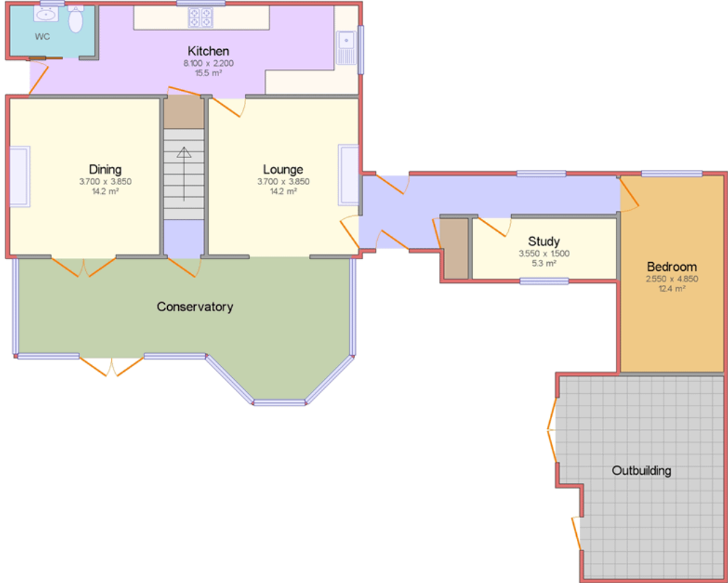
Ground Floor Gross internal area: 160.8 m 2 (1730.4 ft 2 ) Gross internal area: 102 m 2 (House Only)
