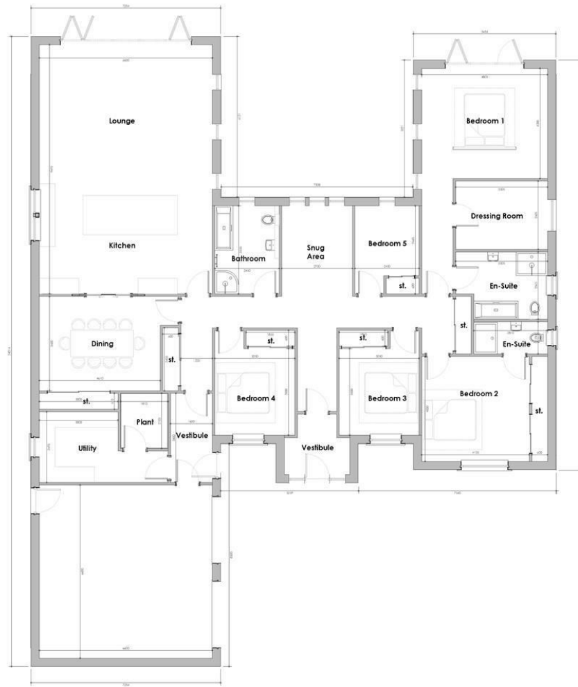
Floor Plan Floor Area Inc Storage - 256.1m 2 Floor Area Inc Garage - 295.7m 2
