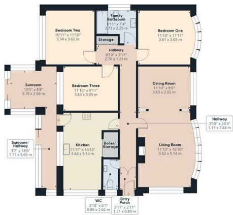
Ground Floor Building 1
