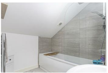
The en suite comprises a panelled bath with a curved shower screen, a waterfall style shower fitting and a hand-held attachment, a pedestal wash hand basin and a low-level WC. Around the bath is full height tiling, with suitable tiling to the rest of the walls. There is ceiling downlighting, an extractor fan and an upright chrome ladder style radiator.
