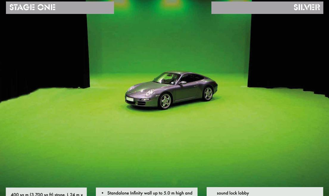
400 sq m (3,700 sq ft) stage, L 24 m  $\times$ W 18 m x H 6.5 dimensions, 3 phase power with 200 amos per phase and single phase power.
