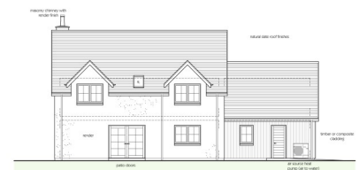
rear (north) elevation
