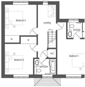
PROPOSED FIRST FLOOR PLAN SCALE 1:50
