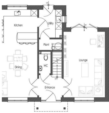
PROPOSED GROUND FLOOR PLAN SCALE 1:50
