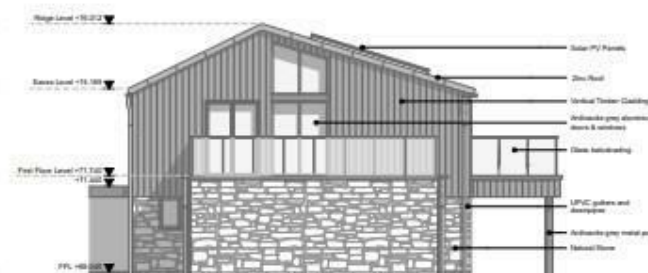
PROPOSED SOUTH ELEVATION 1:100
