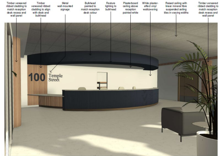
View from Lobby to Reception Desk
