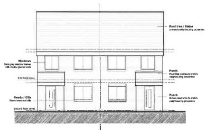
① Proposed Front Elevation Scale 1:100 @ A1
