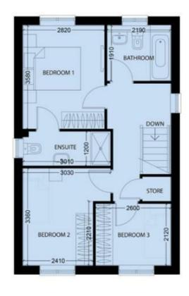
Bedroom 1 3580mm x 2820mm x 3010mm x 1200mm 3010mm x 3030mm x 3030mm x 3030mm x 3030mm x 2600mm x 2120mm a 2190mm x 1910mm
