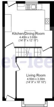
Ground Floor Plan Floor area 37.0 sq. m. (398 sq. ft.) approx
