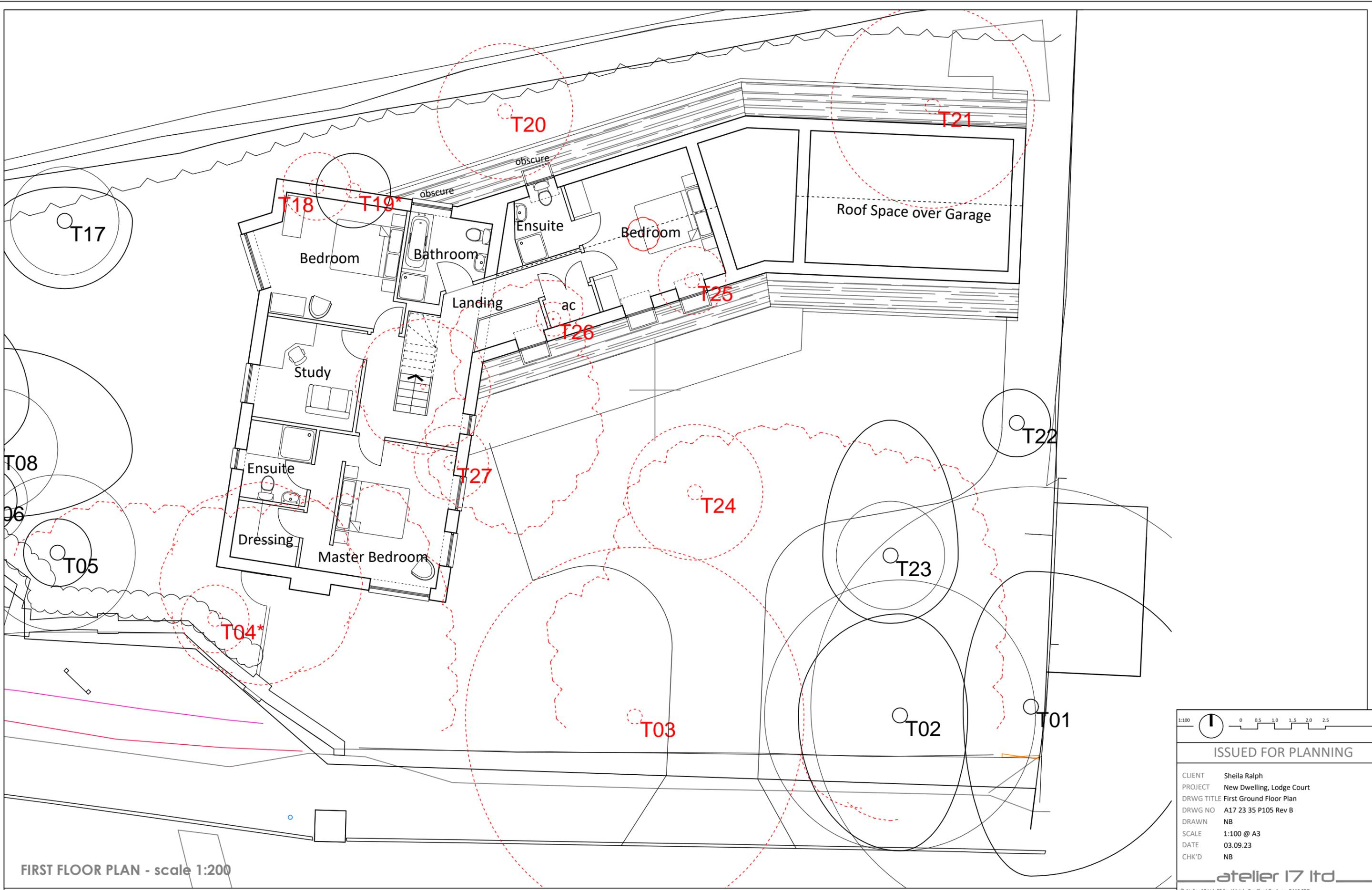
FIRST FLOOR PLAN - scale 1:200
