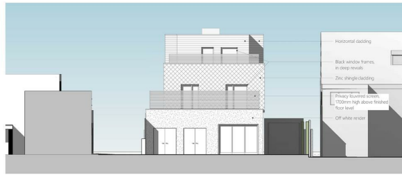
2. Proposed West Elevation scale 1: 100
