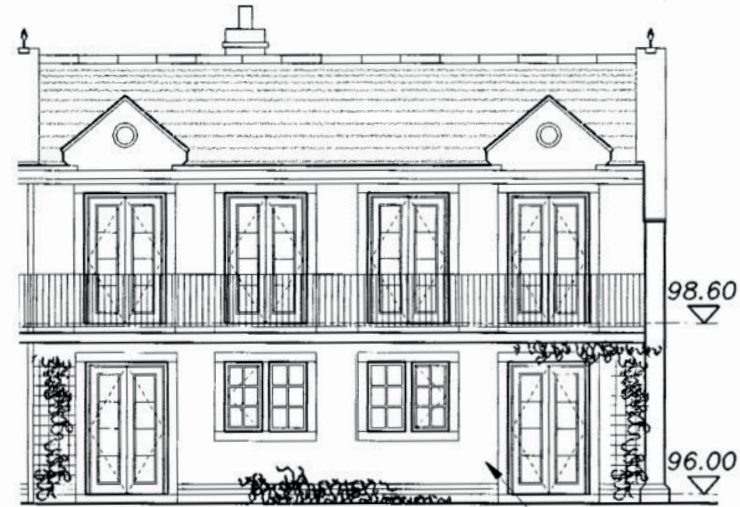
SOUTH WEST ELEVATION. TO BURNLEY ROAD natural coursed stone walling.
