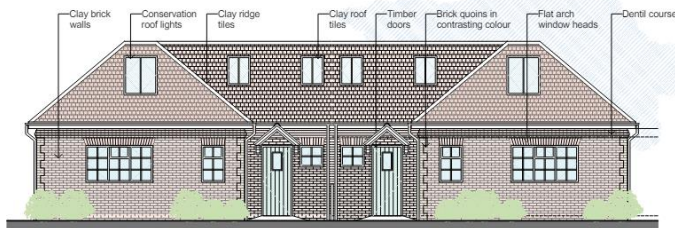
Front Elevation, South East
