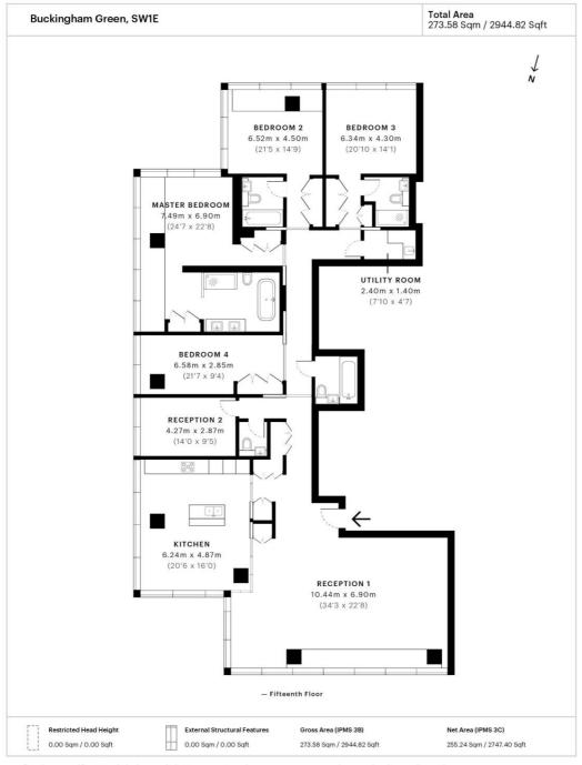
Spec floor plan captured for JLL, Knightsbridge on 03/12/2018 using 79,001,514 laser scan points, accurate to 4/- 3cm. Produced in accordance with Royal Institution of Chartered Surveyors Property Measurement Standards, incorporating International Property Measurement Standard (IPMS). If you intend to rely on any measurement in a transaction you should perform your own checks. Plot/Gardens illustrative only and excluded from all area calculations. Specify: 5c013da81ablad19abd11954
