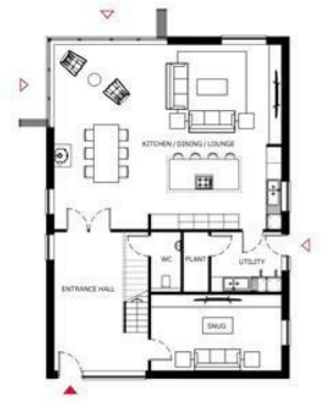
PROPOSED GROUND FLOOR PLAN 1:100 GFA: 116m 2 / 1270 ft 2 GCA: 132m 2 / 1420 ft 2
