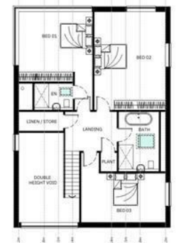
PROPOSED FIRST FLOOR PLAN 1:100 GFA: 98.5m 2 / 1060 ft 2 GCA: 132m 2 / 1420 ft 2
