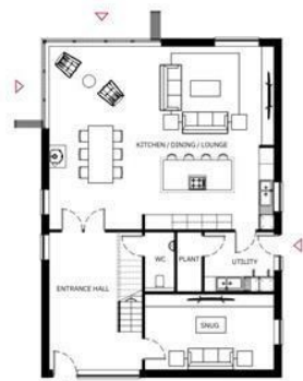
PROPOSED GROUND FLOOR PLAN GFA: 116m 2 / 1270 ft 2 GCA: 132m 2 / 1420 ft 2
