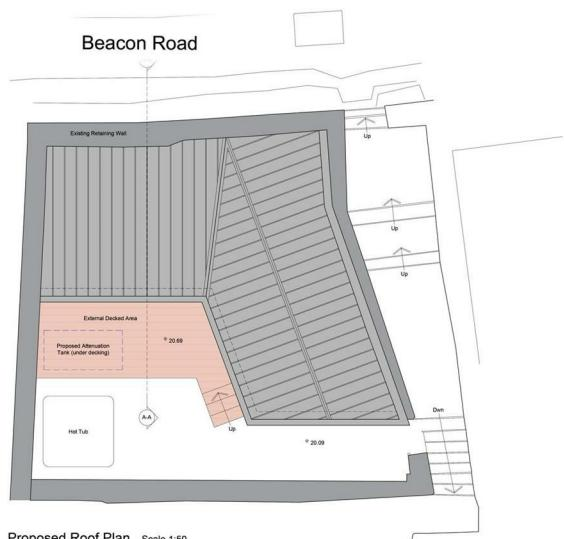
Proposed Roof Plan Scale 1:50
