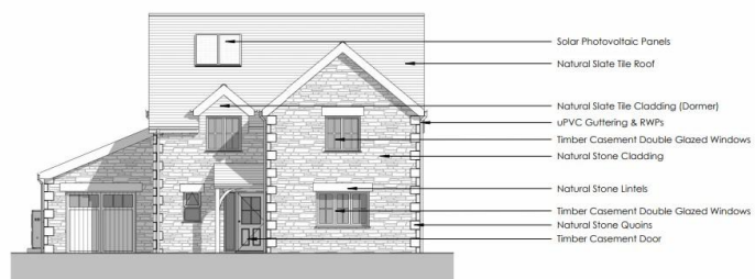
1 South West Elevation 1 : 100
