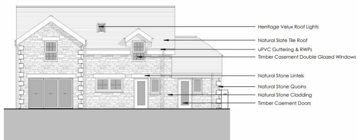
3 North West Elevation 1 : 100
