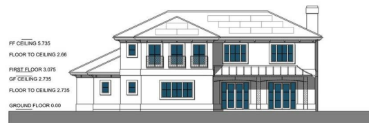
SOUTH WEST ELEVATION
