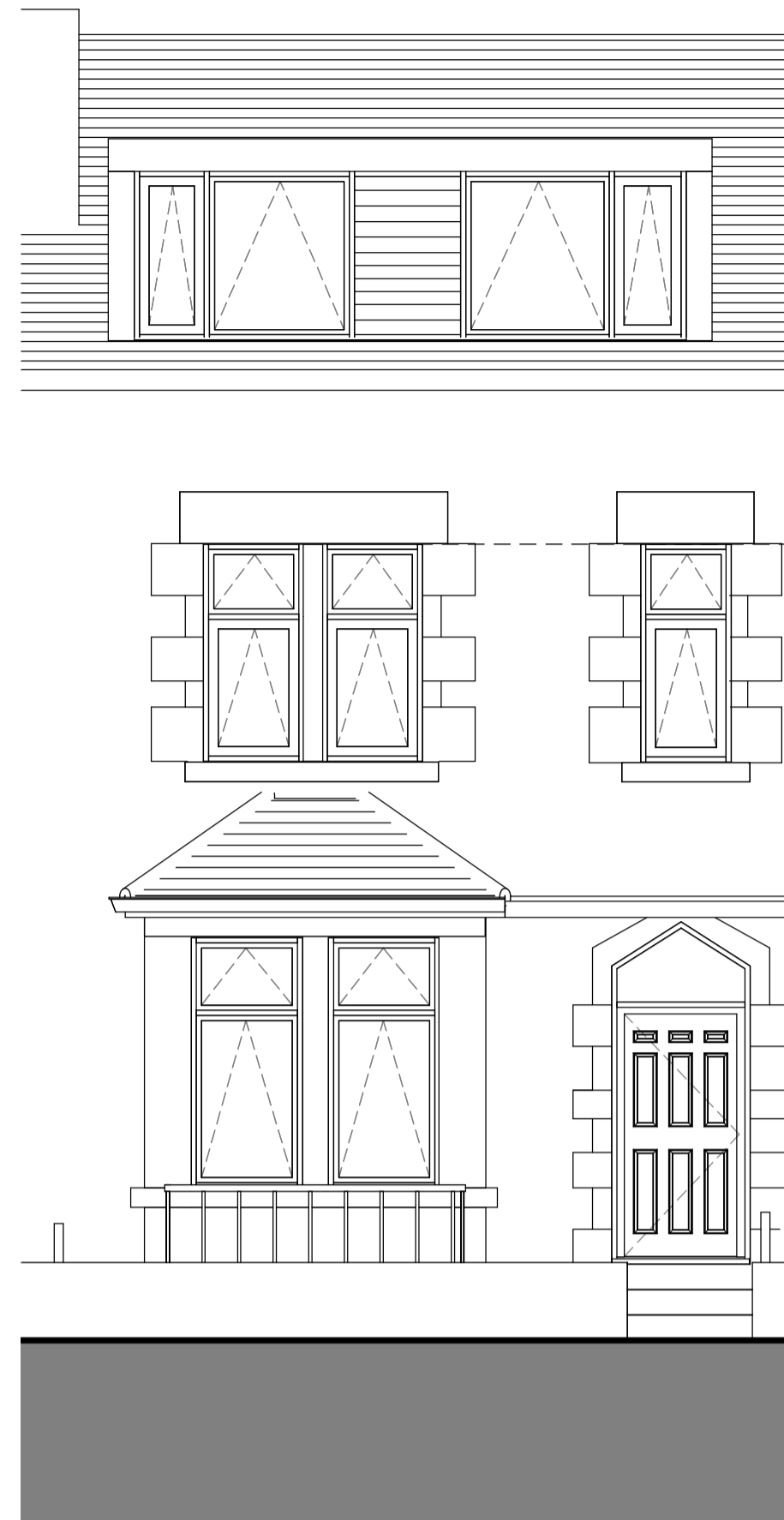
PROPOSED FRONT ELEVATION 1 : 50
