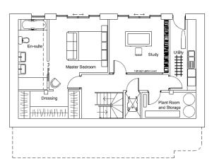
Proposed Lower Floor Plan 1:100 scale 0m 2m 1:100 Scale Bar
